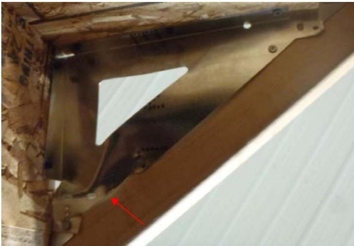
Ultimate load failure mode
