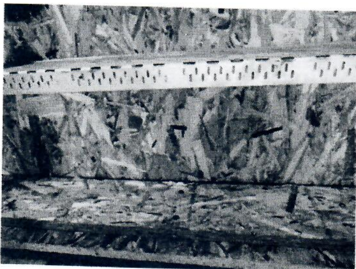
Gangnail brace after 1,000,000+ cycles
